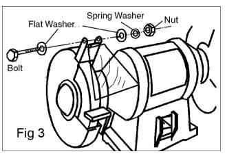
holes in the base. Do not overtighten the mounting bolts as this could damage the plastic base.
